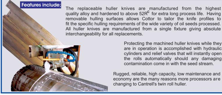
removable hulling surfaces allows Cottor to tailor the knife profiles to fit the specific hulling requirements of the wide variety of oil seeds processed. All huller knives are manufactured from a single fixture giving absolute
