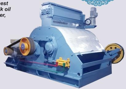
The heart of the hulling process is the twin, rugged rolls equipped with removable huller knives. These twin rolls are driven at a ratio to enhance the cutting process thus minimizing the amount of uncut and recycle seed. This ratio combined with a spiral lead on the cutting edges allows the highest percentage of open "hulled" seed available to the separation room.
